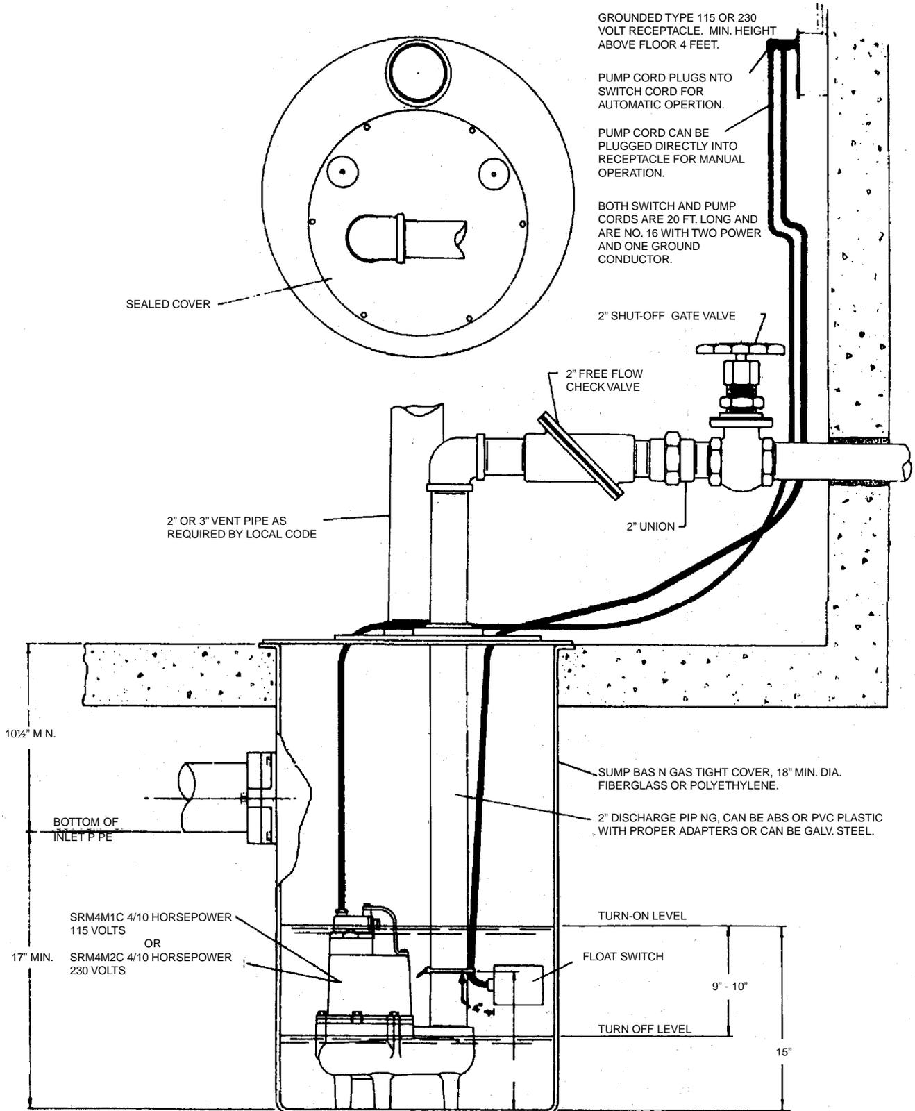
**CAUTION: FOR ANY WORK ON PUMP OR SWITCH, ALWAYS UNPLUG POWER CORD. DO NOT JUST TURN OFF CIRCUIT BREAKER OR UNSCREW FUSE.**
